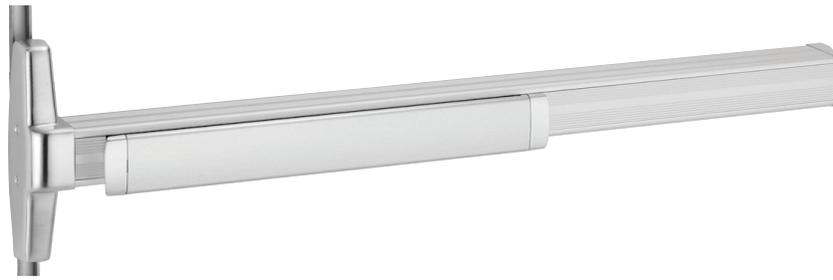
**3348A and 3548A** for hollow metal single and double doors, UL listed for panic exit hardware. Devices are ANSI A156.3 – 2008 Grade 1. The 3548A has a smooth mechanism case and the 3348A has grooved case. The concealed vertical rod device is non-handed except when the SS (Signal Switch) option is used.
