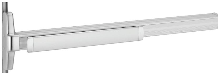
**3348A-F and 3548A-F** for hollow metal single and double doors up to 8' x 10' (2438mm x 2540mm), UL listed for fire exit hardware. See Additional information section of the catalog for detailed information on UL listed fire exit hardware label and door opening size information. Devices are ANSI A156.3 – 2008 Grade 1. The 3548A-F has a smooth mechanism case and the 3348A-F has grooved case. The concealed vertical rod device is non-handed except when the SS (Signal Switch) option is used.
