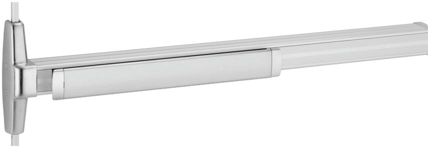
**3327A-F and 3527A-F** for all types of double doors up to 8' x 10' (2438mm x 2540mm), UL listed for Fire Exit Hardware. See Additional information section of the catalog for detailed information on UL listed fire exit hardware label and door opening size information. Devices are ANSI A156.3 – 2008 Grade 1. The 3527A-F has a smooth mechanism case and the 3327A-F has grooved case. The surface vertical rod device is non-handed except when the SS (Signal Switch) option is used.
