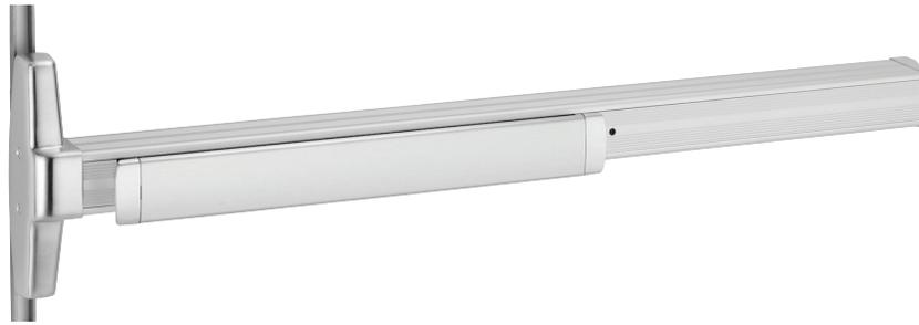
**3347A and 3547A** for all types of single and double doors, UL listed for panic exit hardware. Devices are ANSI A156.3 – 2008 Grade 1. The 3547A has a smooth mechanism case and the 3347A has grooved case. The concealed vertical rod device is non-handed except when the SS (signal switch) option is used.
