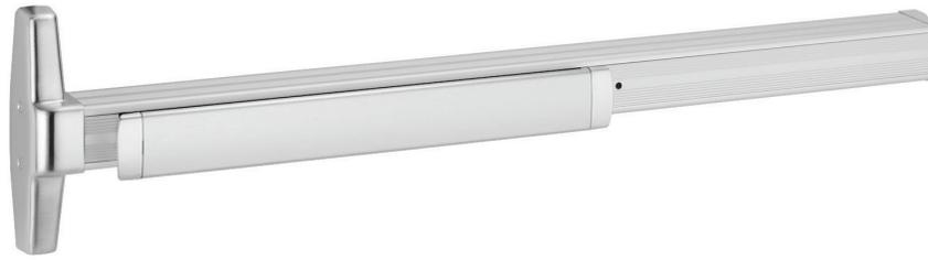
**3350AWDC and 3550AWDC** for use on single and double wood doors, UL listed for panic exit hardware. Devices are ANSI A156.3 – 2008 Grade 1. The 3549A has a smooth mechanism case and the 3350AWDC has grooved case. The concealed vertical cable device is non-handed except when the SS (signal switch) option is used.
