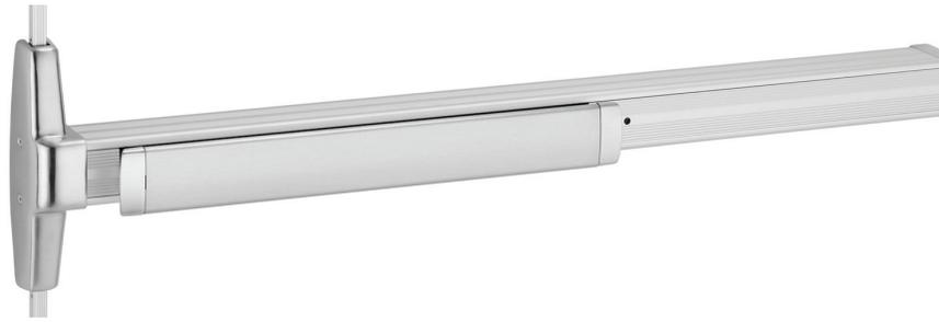
**3327A and 3527A** for all types of single and double doors, UL listed for panic exit hardware. Devices are ANSI A156.3 – 2008 Grade 1. The 3527A has a smooth mechanism case and the 3327A has grooved case. The surface vertical rod device is non-handed except when the SS (signal switch) option is used.
