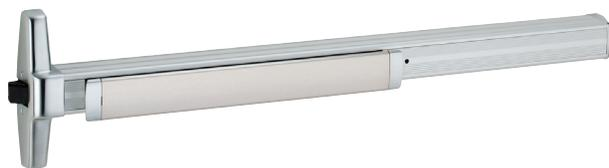
The PN feature provides remote latch bolt retraction in hazardous areas where electrically operated devices would not be permitted. The pneumatic solenoid will retract the latch bolt for momentary or prolonged periods. PN exit devices are particularly suited for use with automatic door operators. The PN feature is available on both Panic and fire exit hardware devices.
